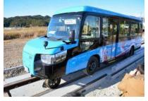
on the road but its steel wheels, which are in its underbelly, descend when it hits the rail tracks.
