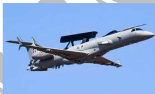
ii. The Netra, an **Airborne Early Warning and Control (AEWC) aircraft**, is useful for surveillance, tracking, identification and classification of airborne and sea surface targets and is useful in detecting incoming ballistic missile threats.
