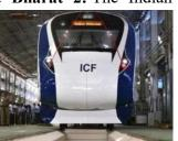
• According to the Ministry of Railways, Vande Bharat 2 According to ministry, Vande Bharat 2 will have further improvements and developments, including a faster 0 to 100 Kmph time of just 52 seconds, a top speed of 180 Kmph, a lighter weight of 392 tonnes, and WI-FI content that is available when needed.
